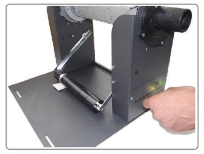
6. Move the tension arm about 2/3 of the way to the top and insert the clip to press the button again. The green LED will be flashing.
